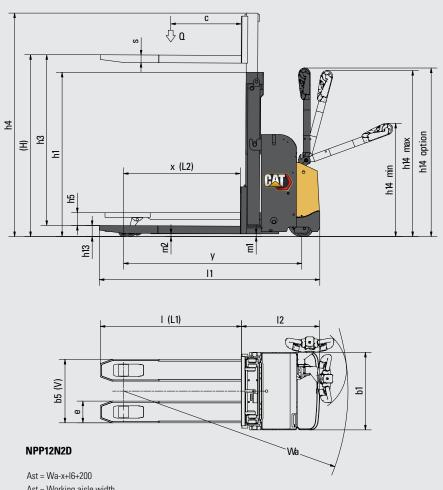
Ast = Working aisle width Wa = Turning radius a = Safety clearance (200 mm) I6 = Pallet length
