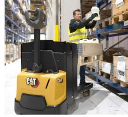
The NPP20N3E is equipped with lifting forks (730 mm height) that offer an ergonomic position for loading and unloading items with minimal physical strain.
