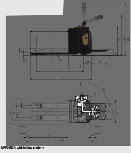
Ast = Wa-x+l6+200 Ast = Working aisle width Wa = Turning radius a = Safety clearance (200 mm) I6 = Pallet length
