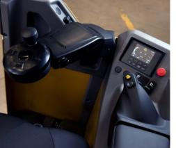
User-friendly controls include fingertip hydraulic levers, with an adjustable armrest, and a positionally adjustable mini steering wheel. The truck's easy and precise manoeuvring and load handling are ideal for a variety of applications and tasks. They include general warehouse work, as well as material flow in factories.
